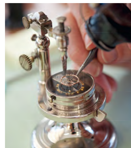
Counting of the mainspring/ determination of the length
