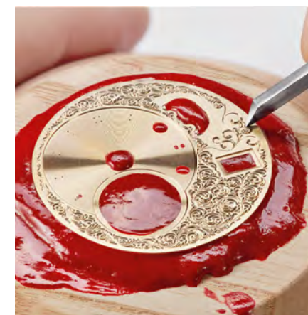
Manual engraving of the PanoLunar Tourbillon
