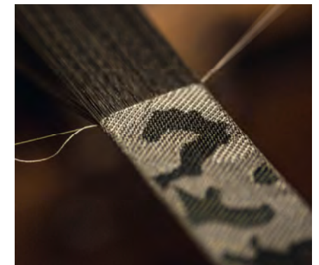
Weaving of the Heritage Ranger textile strap on the antique Jacquard weaving loom
