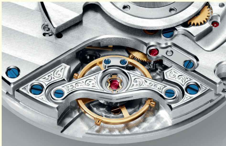
Just like in the CW3, the balance is fitted with a freely swinging balance-spring without a regulator for improvement of the rate performance
