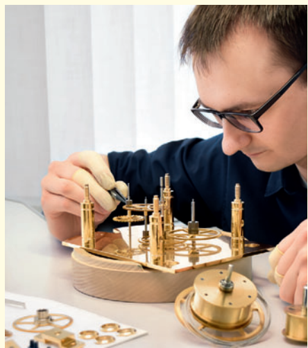
Watchmaker Robert Flöter during assembly of the movement
